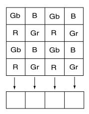
The bottom left pixel is the first signal output
